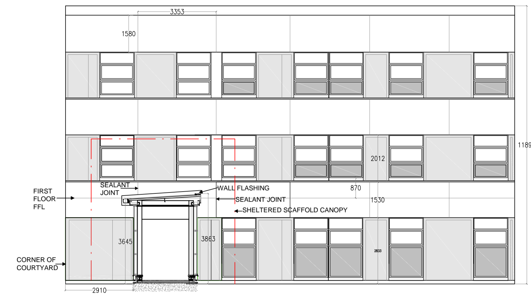
EXISTING ELEVATION C 1:100
