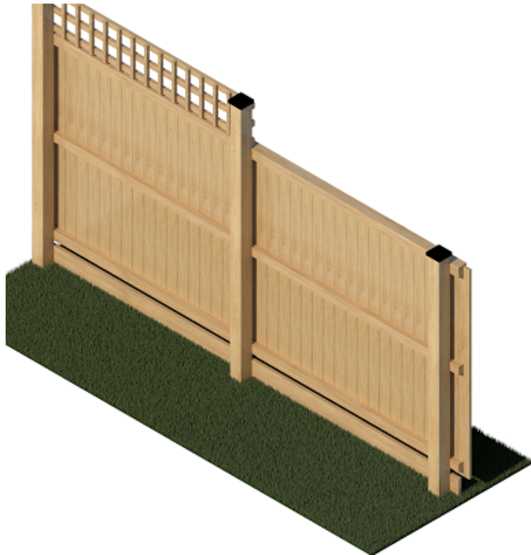
Trellis formed from 44 x 25mm horizontal and 25 x 25mm vertical members.
