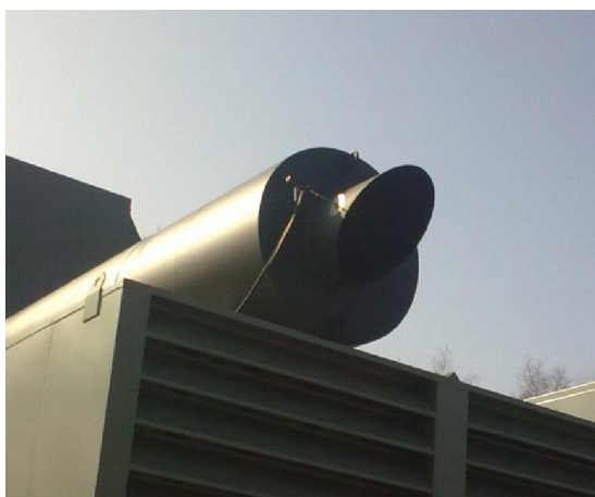
Figure 1: Testo 350 XL probe in the exhaust of the Perkins 4012-46TAG 3A
