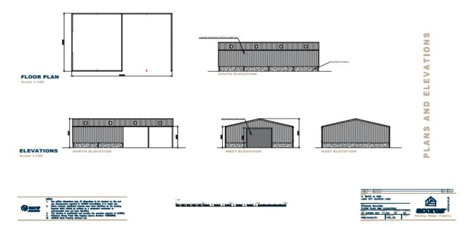
The applicant seeks permission for the erection of an agricultural storage building to measure 12.3 meters by 18.3 meters with a height to the eaves of 4.5 meters and 6.15 meters to the ridge. The materials used will be concrete panels with box profile steel sheeting (Juniper Green) above. The roof covering will be box profile steel sheeting (Juniper Green) with clear roof lights.
