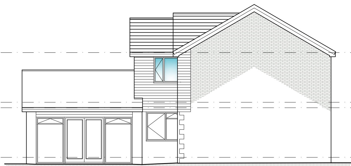
PROPOSED SIDE ELEVATION SCALE 1:100
