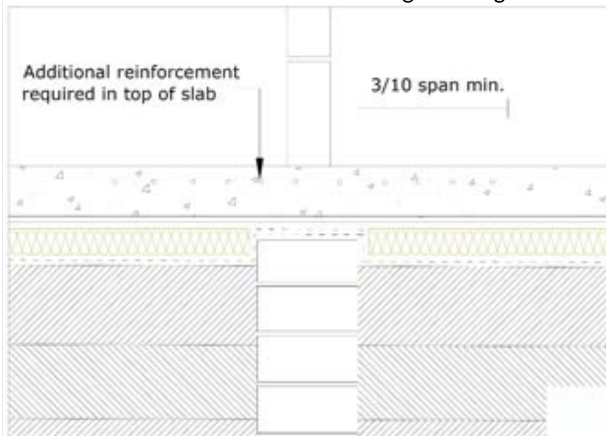
Diagram B57 - Typical slab detail continuous over a wall
