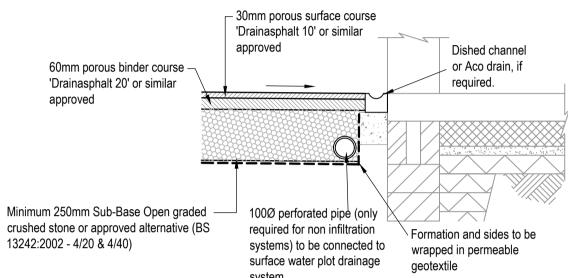
PERMEABLE TARMAC CONSTRUCTION DETAIL (PRIVATE DRIVE FALLING TOWARDS GARAGE/PLOT)
