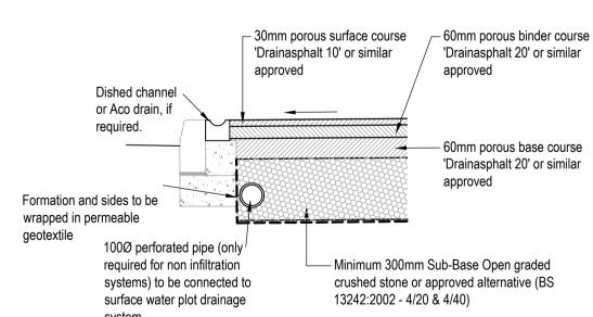
PERMEABLE TARMAC CONSTRUCTION DETAIL (SHARED DRIVE FALLING TOWARDS HIGHWAY)
