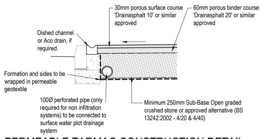
PERMEABLE TARMAC CONSTRUCTION DETAIL (PRIVATE DRIVE FALLING TOWARDS HIGHWAY)
