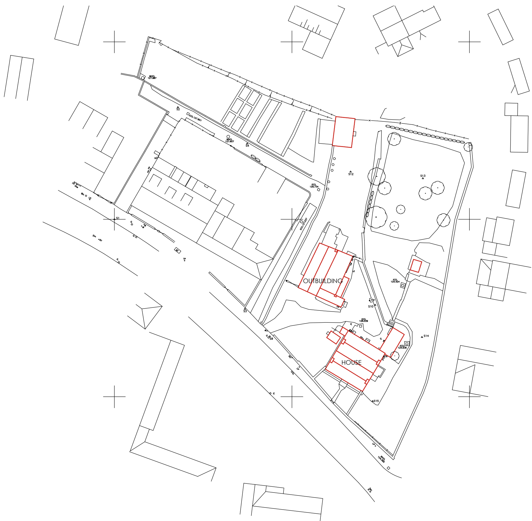
STRUCTURES TO BE DEMOLISHED SCALE 1:500
