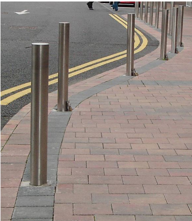
Controlled access for vehicles: Removable bollards
