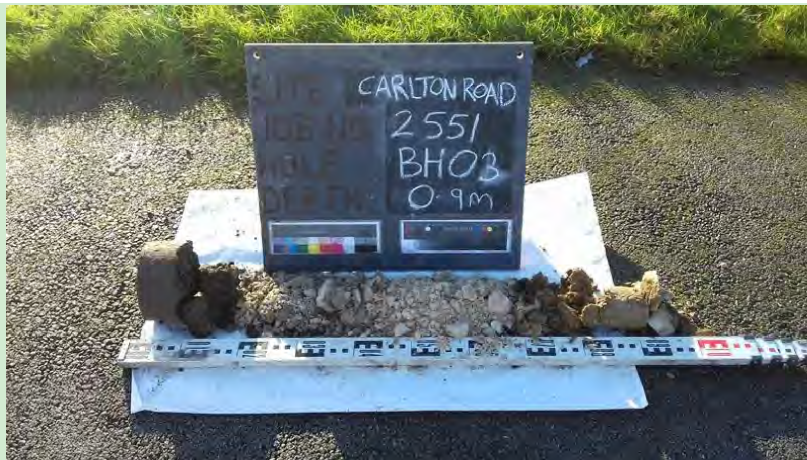
BH03 – final depth 0.9m
