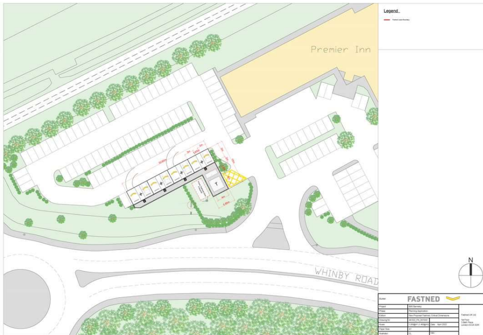
Figure 2.3 Site layout: Dimensions of proposed infrastructure at the existing carpark off Whinby Road
