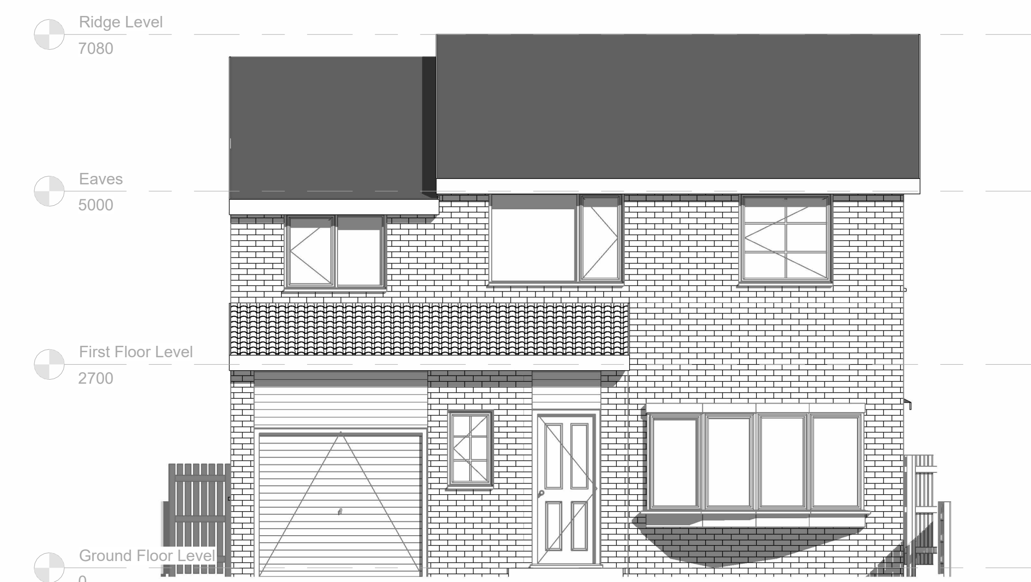
Proposed West Elevation 1 : 50
