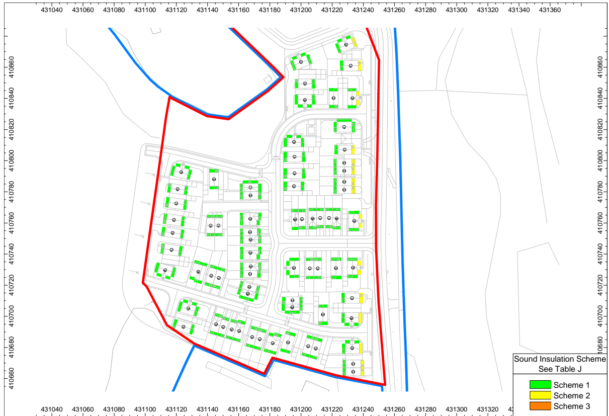
Figure I: Illustration of Sound Insulation Scheme – Site A
