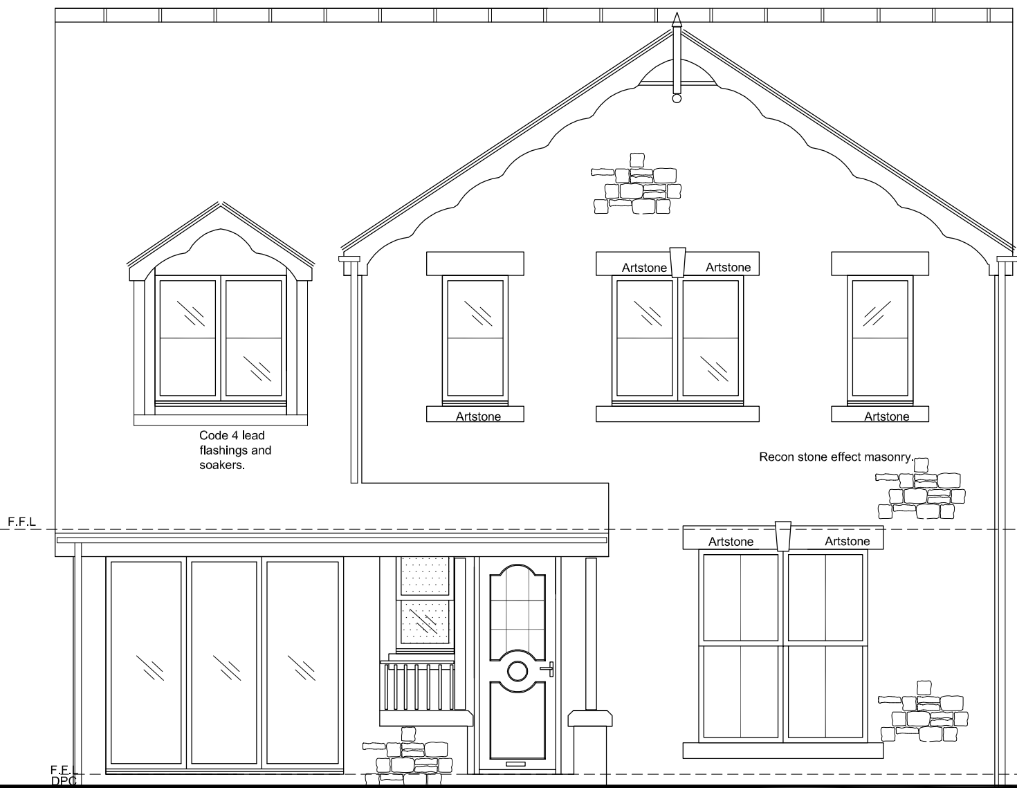
EXISTING FRONT ELEVATION. 1/50
