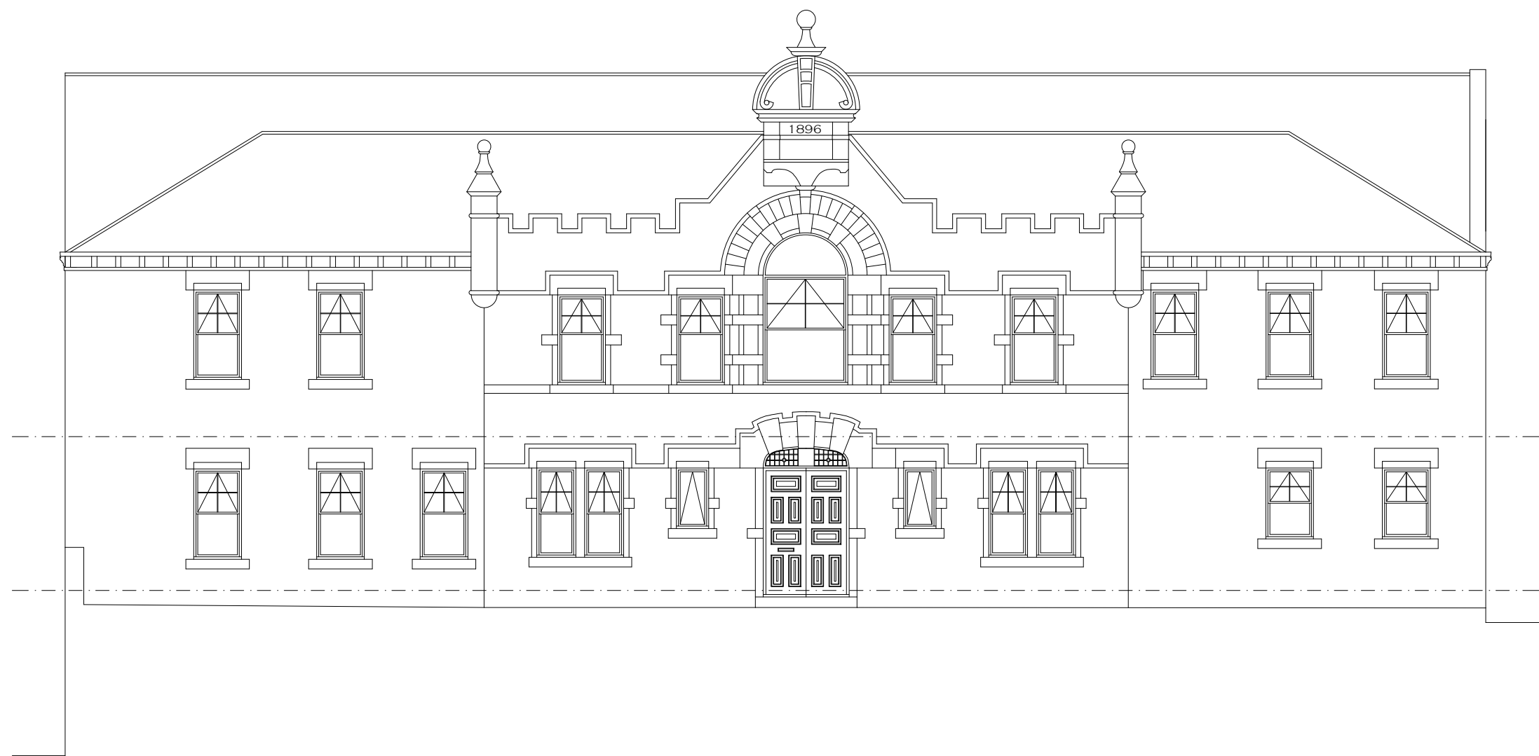
PROPOSED FRONT ELEVATION (EASTGATE) SCALE 1:100
