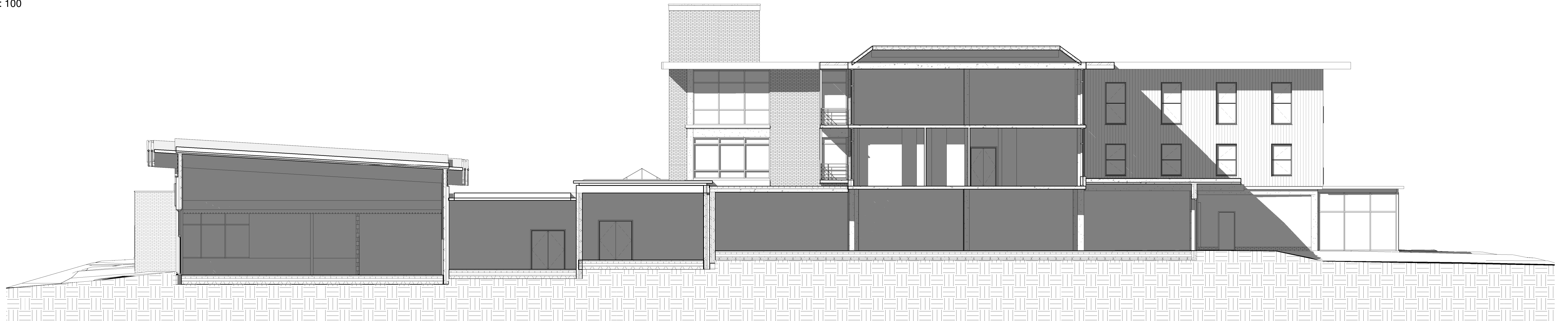
2 Floor Level Section As Proposed 1 : 100
