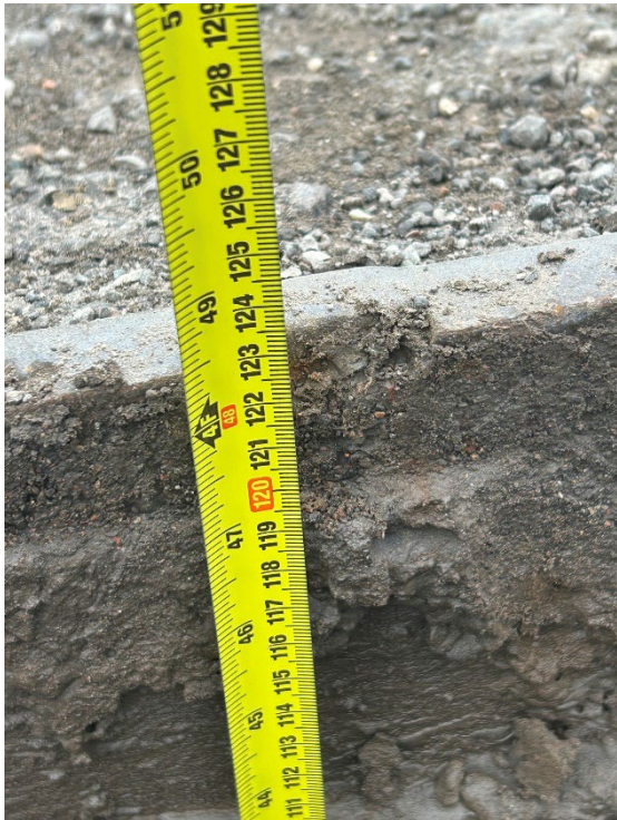
Figure H2 – Tape Measurement Showing 1.22 m Invert
