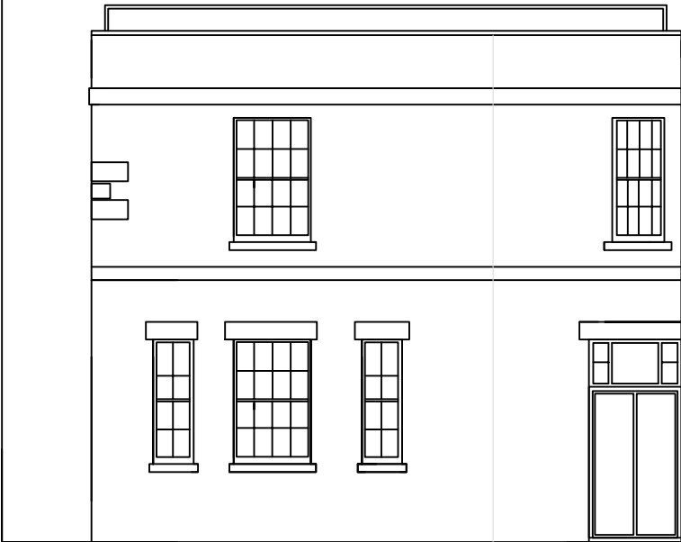
EXISTING SOUTH ELEVATION
