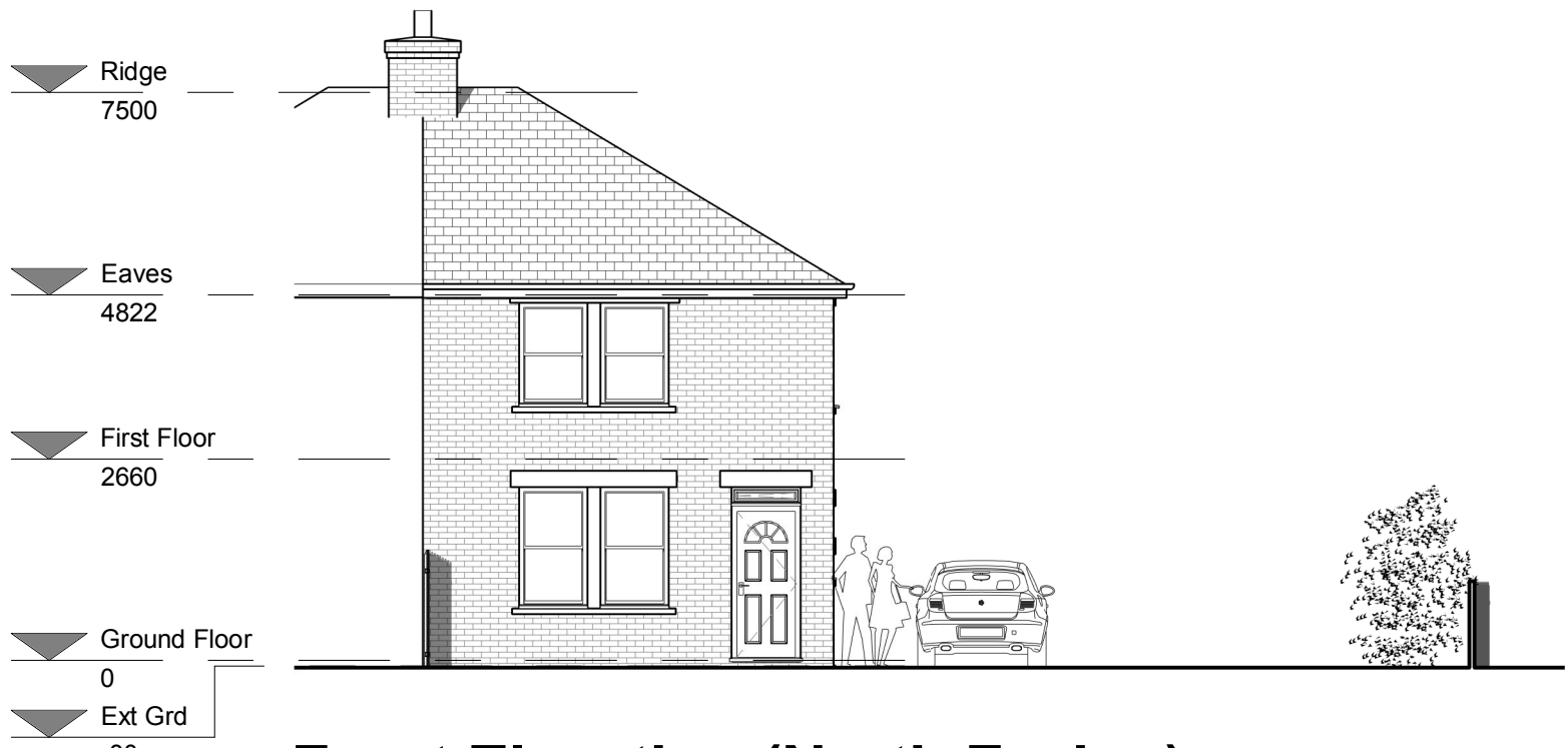
Front Elevation (North Facing)
