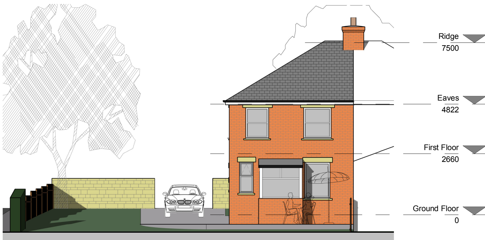
Rear Elevation (South Facing)
