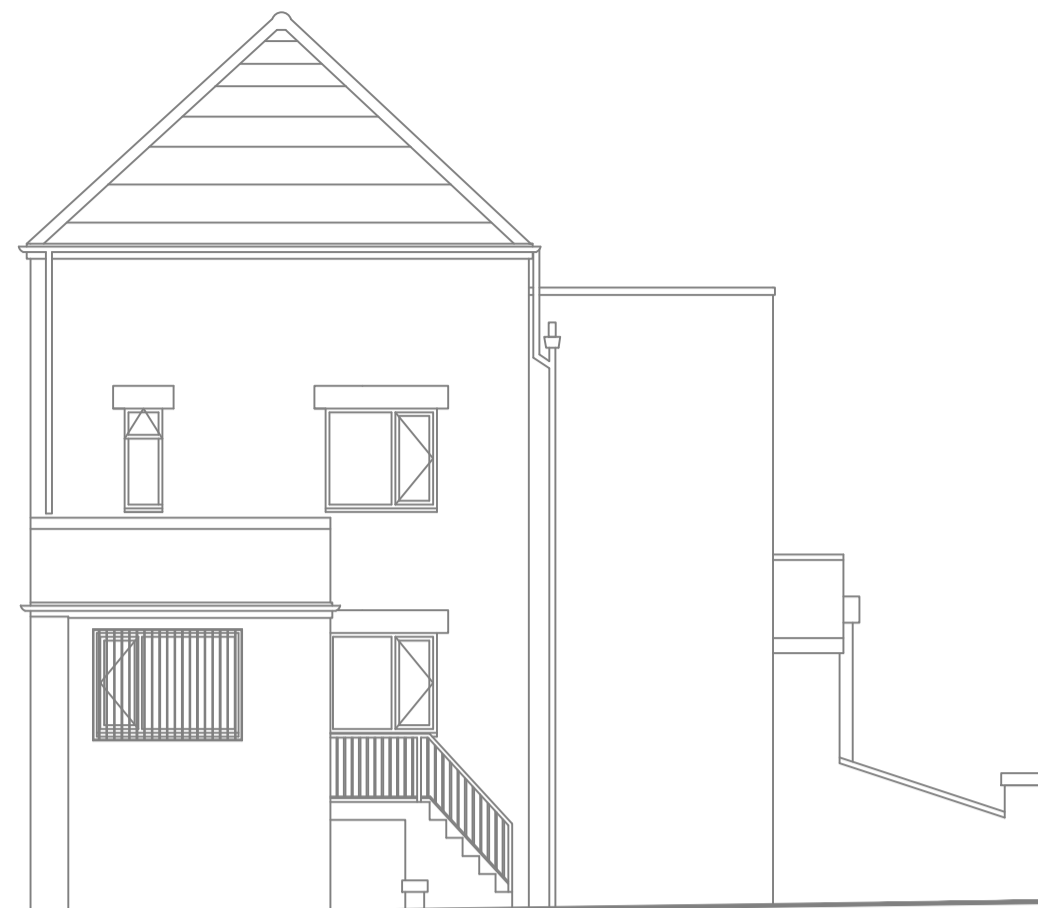
Main Building - Existing Elevation B
