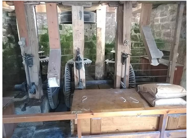
Corn Mill: Mill stones and mechanism
