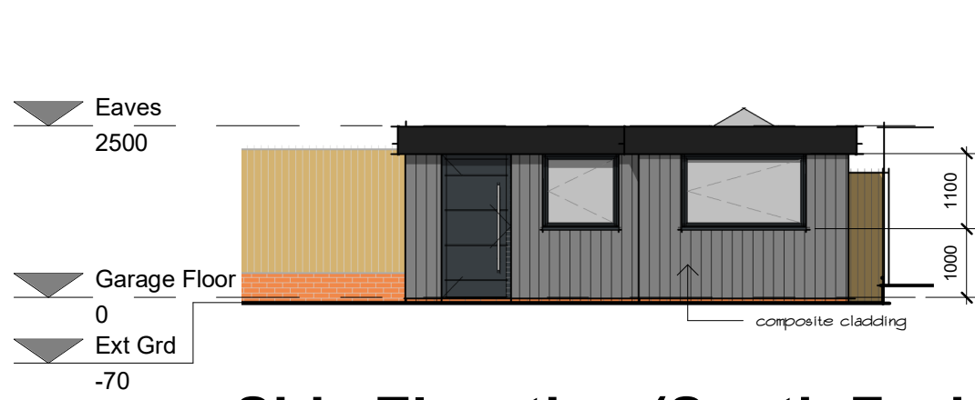
Side Elevation (South Facing) 1 : 100
