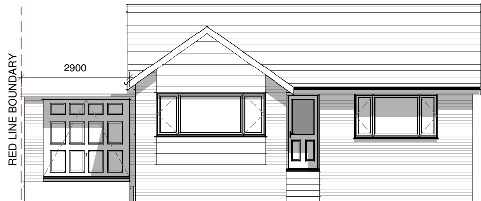
Front Elevation Boundary Identification 1 : 100
