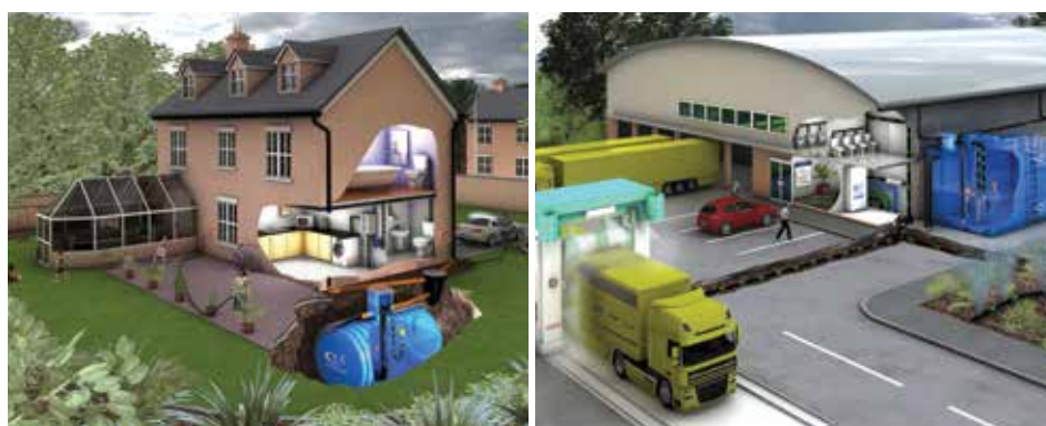
Figure 11.1 Rainwater harvesting storage tanks for domestic and commercial application (courtesy Stormsaver)
