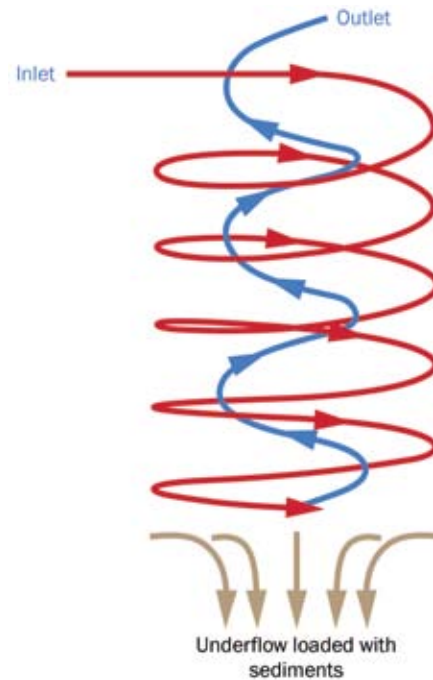
Figure 14.4 Simplified flow pattern in a vortex separator (from NJCAT, 2005)
