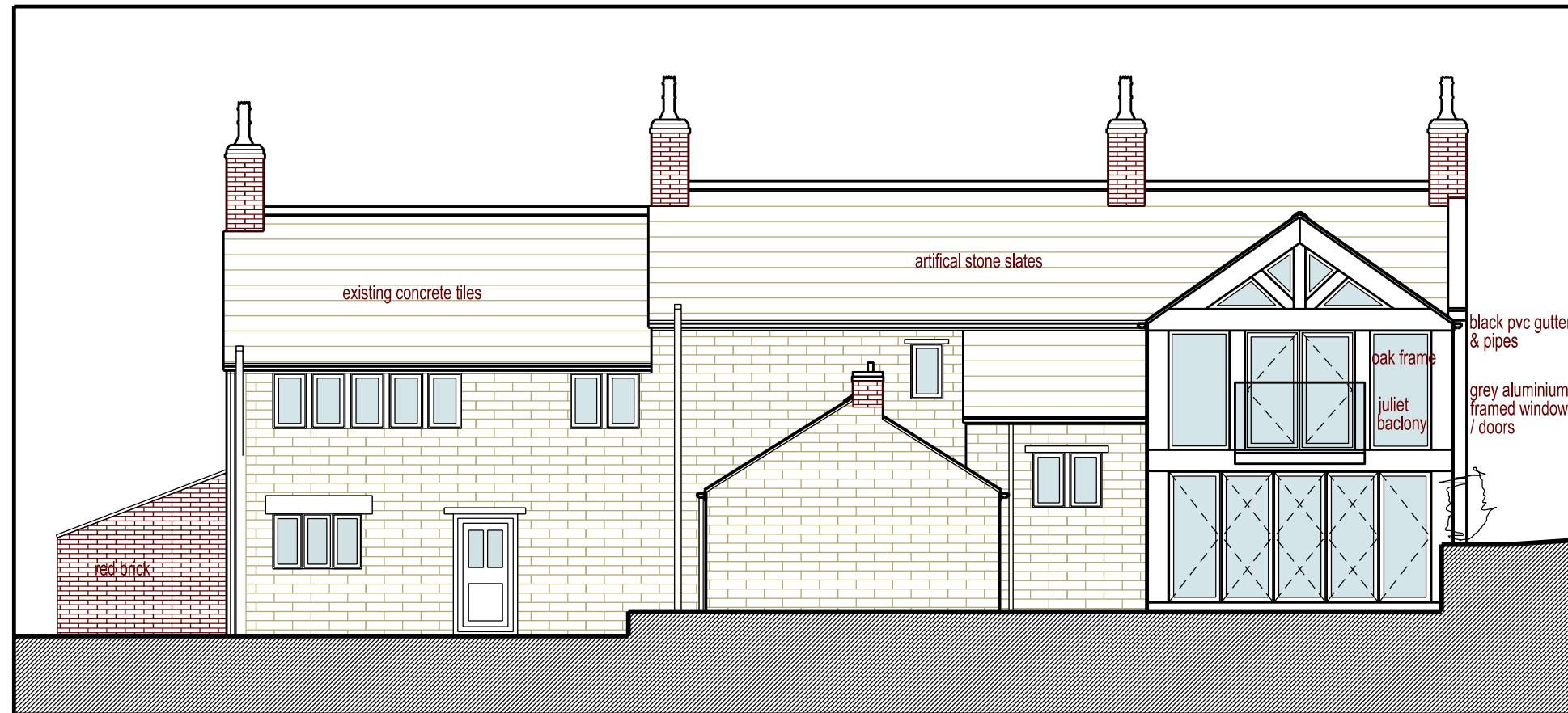
North Elevation - Existing
