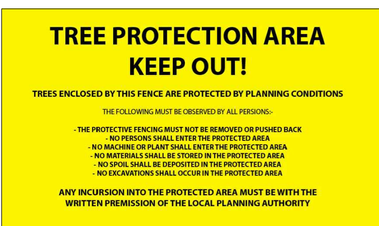
Figure 4 - Typical protection fence signage
