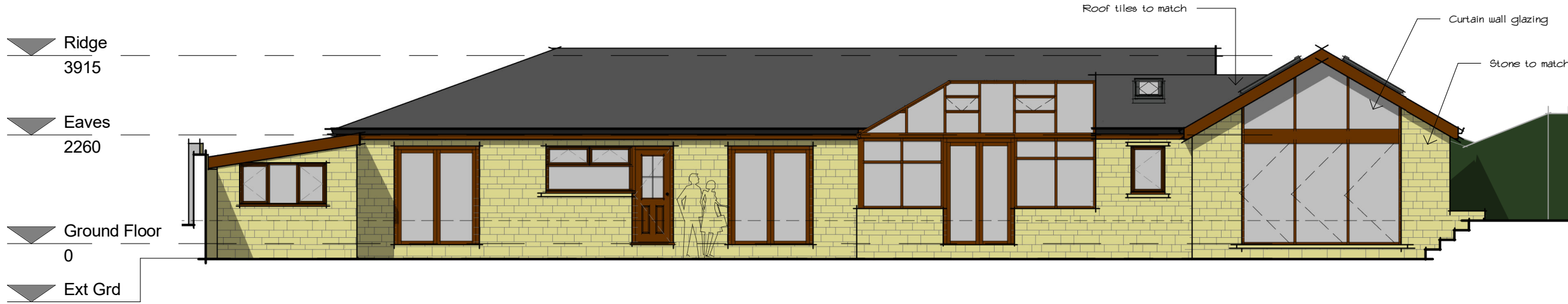
Rear Elevation (South Facing) 1 : 100
