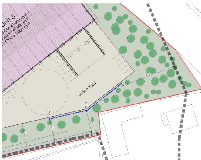
Figure 1 Location of retaining wall
