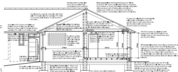
SECTION THRU' UTILITY EXTENSION
