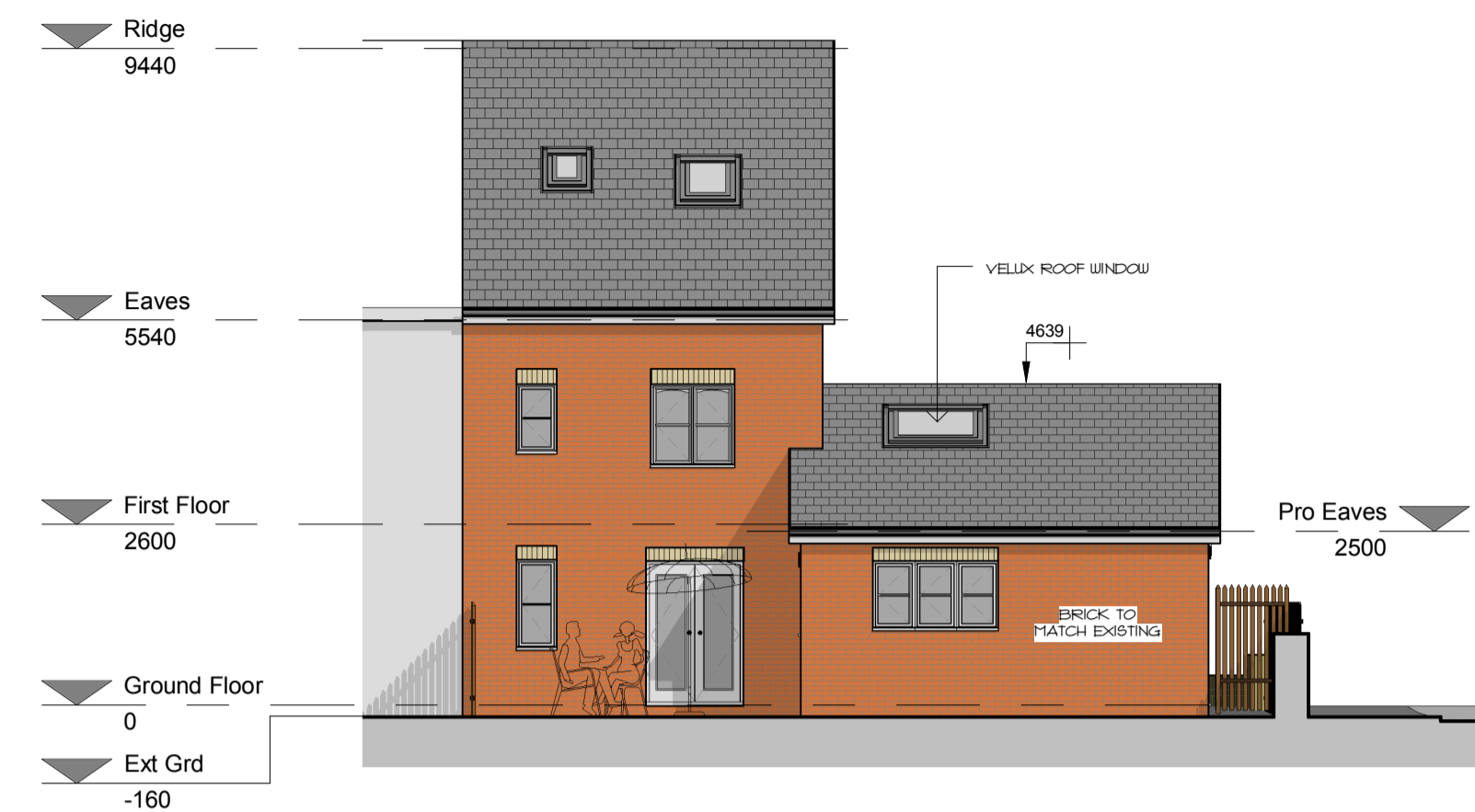
Rear Elevation (South Facing) 1 : 100
