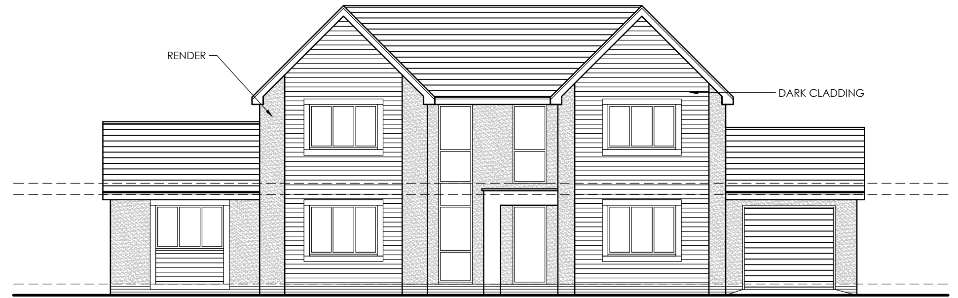
PROPOSED FRONT ELEVATION SCALE 1:100
