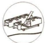
a) Stabilizer strut with base plate secured with ground pins
