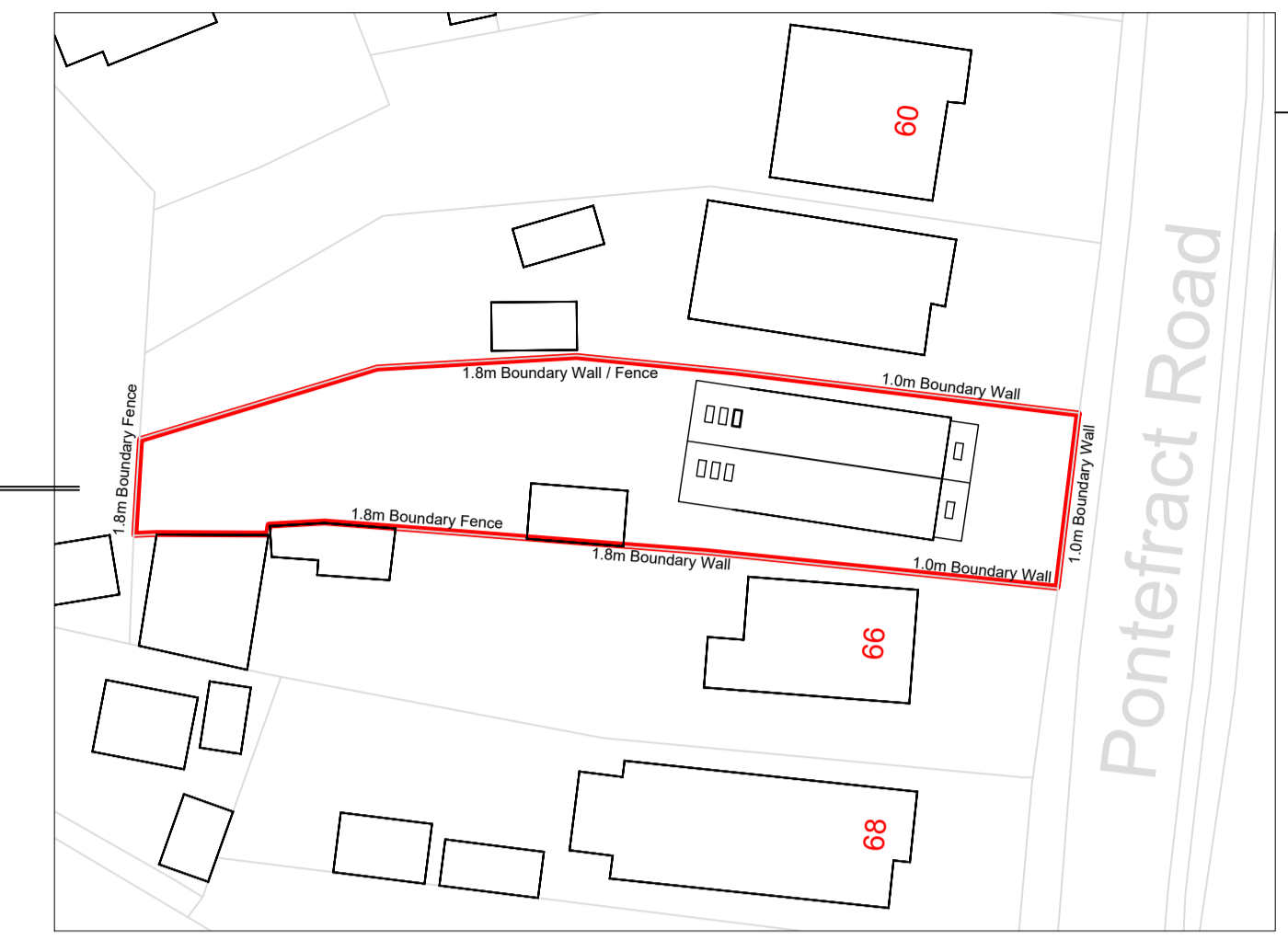
Site Plan as Proposed © Crown copyright and database rights [2022] Ordnance Survey 0100031673 Scale: 0 5m 10m 20m 1:500
