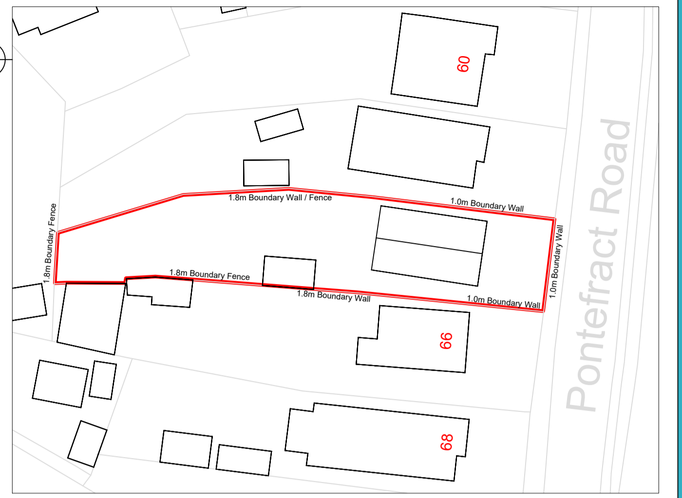
Site Plan as Existing © Crown copyright and database rights [2022] Ordnance Survey 0100031673 Scale: 0 5m 10m 20m 1:500 Land under client ownership
