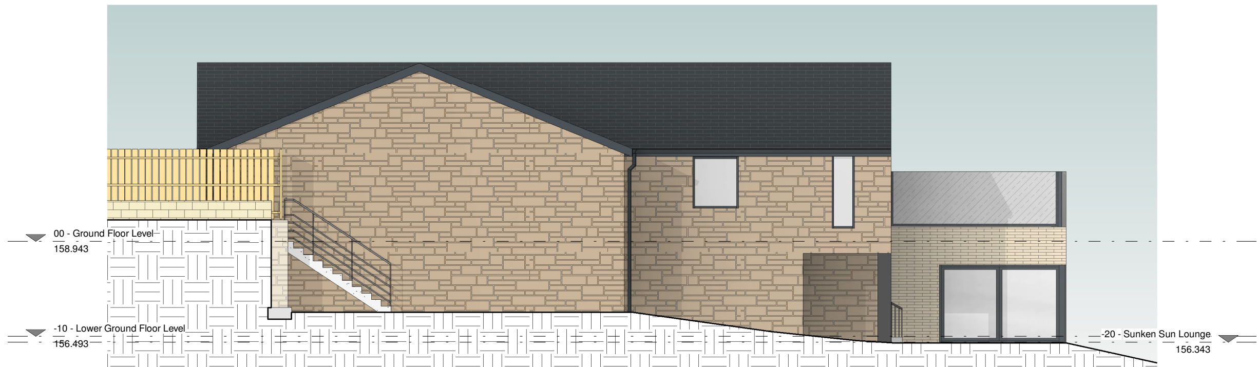
Proposed East Elevation Scale: 1 : 100
