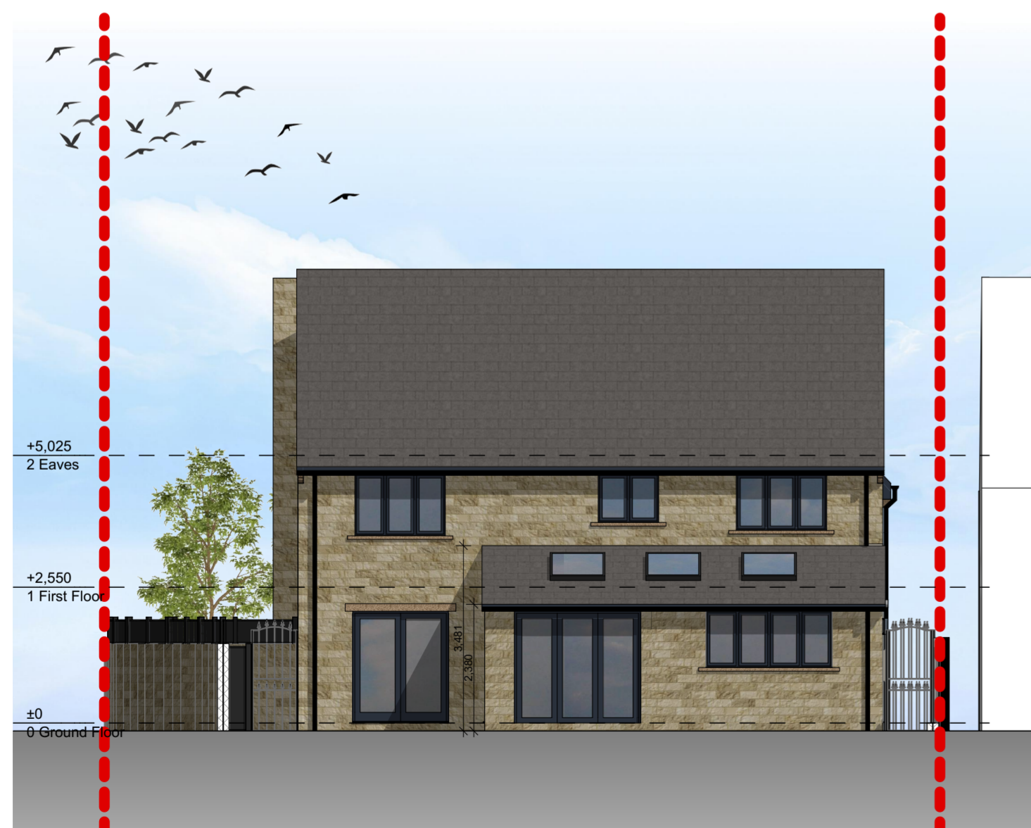
Proposed SE Elevation
