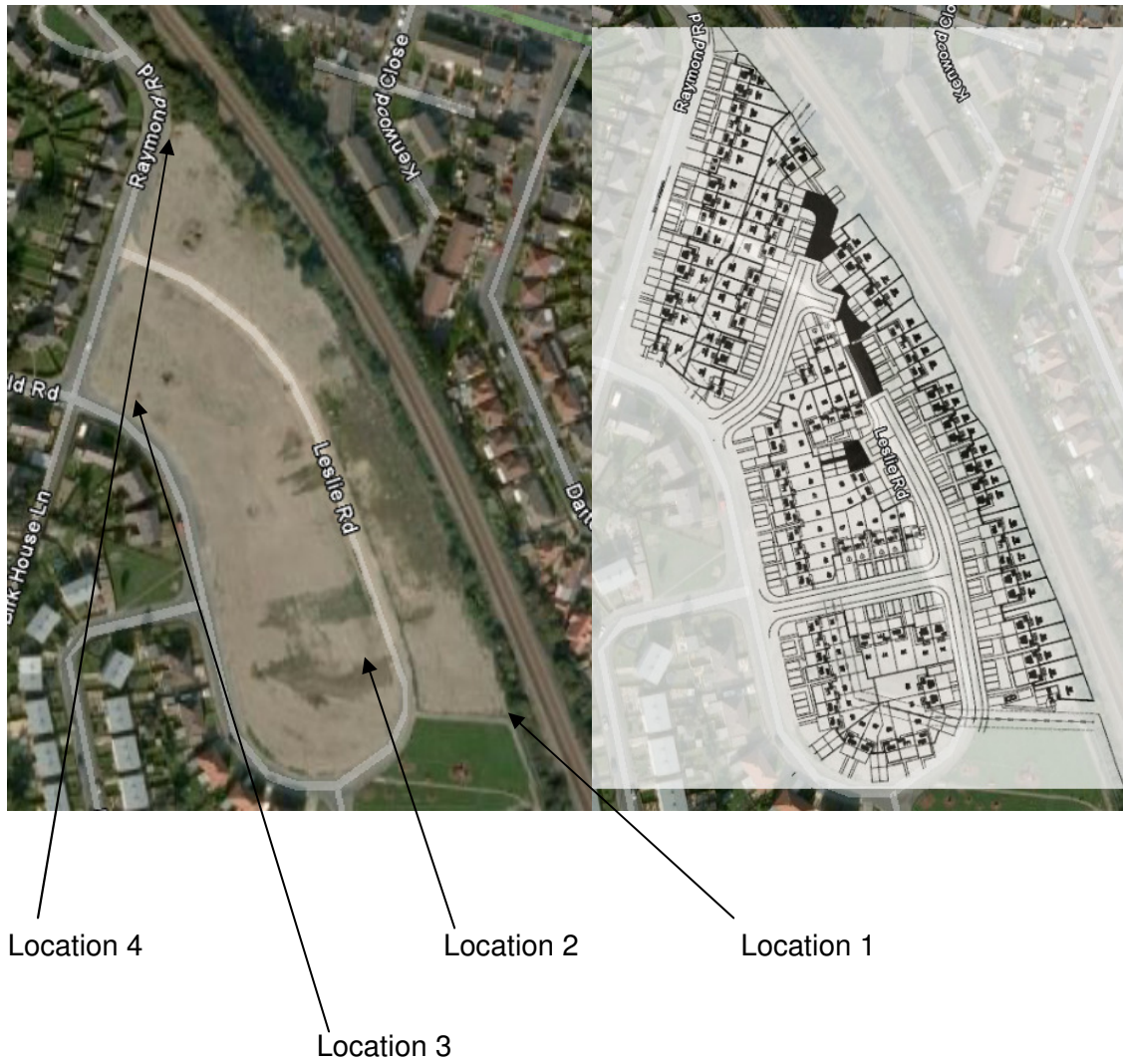
FIGURE 1 – POSSIBLE SITE LAYOUT SHOWING NOISE MONITORING LOCATIONS
