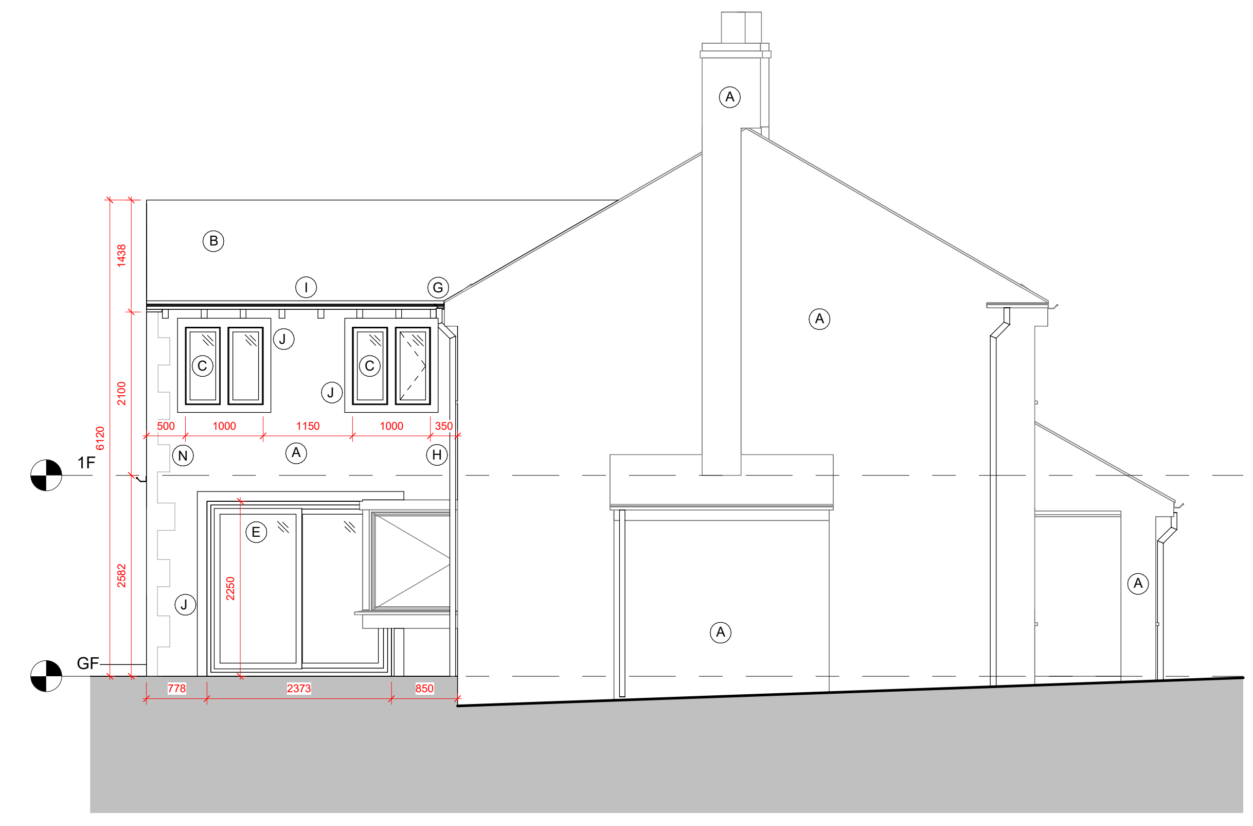
4 Proposed East Elevation. 1 : 50
