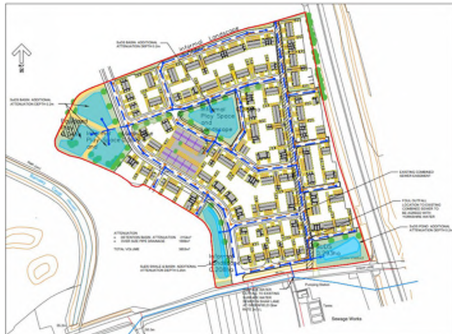
Figure 10 – Indicative Surface Water Drainage Strategy
