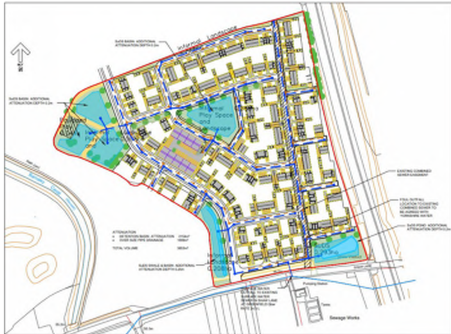
Figure 12 – Indicative Foul Water Drainage Strategy
