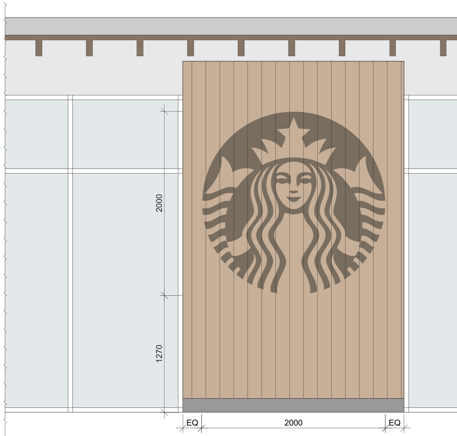
M 2000mm dia. Hand Painted Siren Logo - Scale 1:20 COLOUR - RAL 7013 - on previously approved cladding finish
