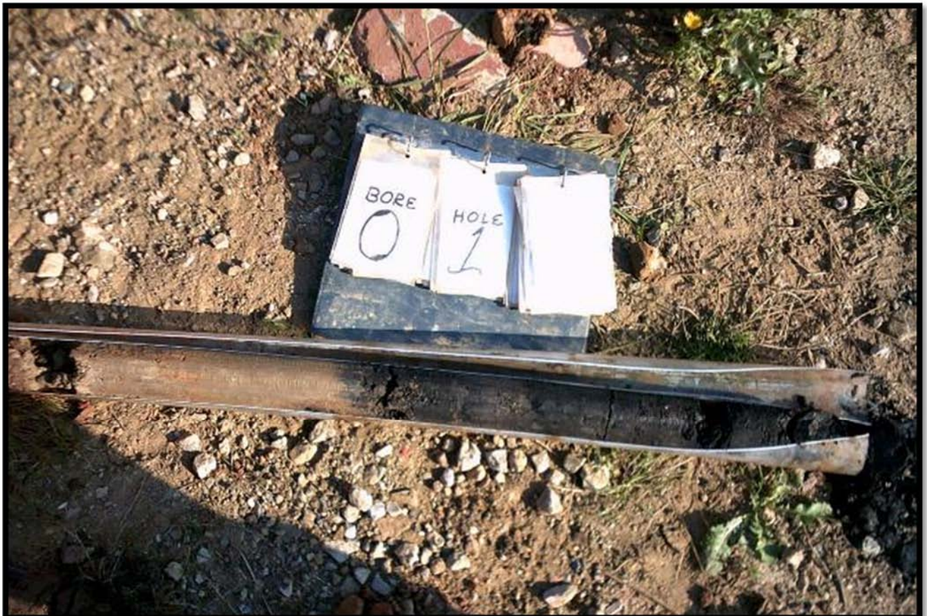
U: Dirty coal at the base of window sample borehole WS01.
