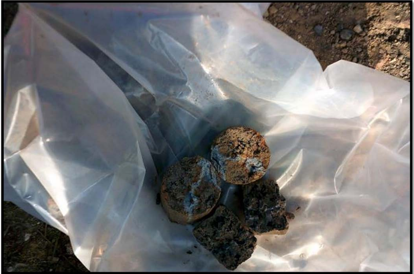
T: Sandy gravelly clay of completely weathered bedrock.
