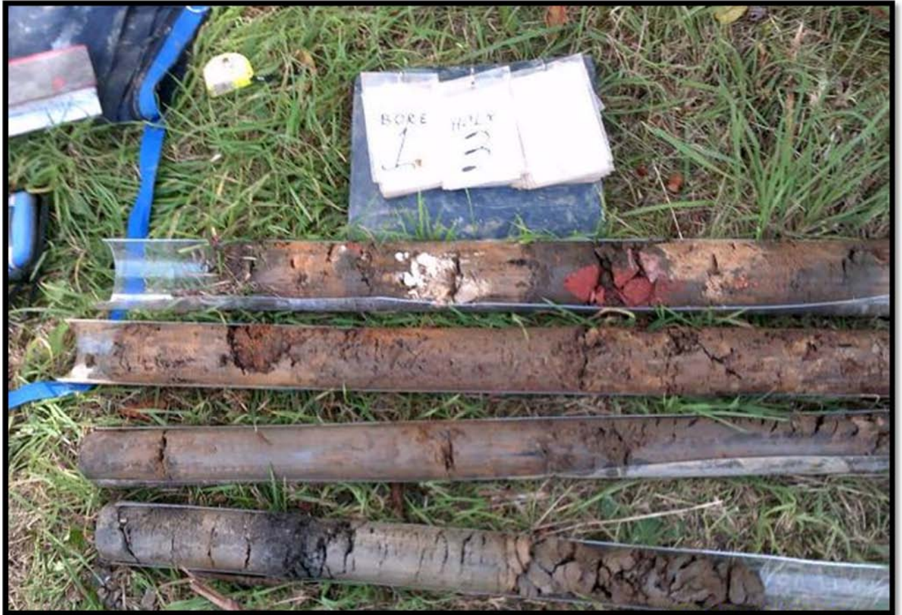
Z: Cores from WS13 showing a typical soil profile with clay grading to mudstone.
