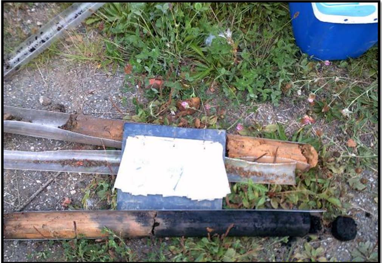
X: Cores from window sample borehole WS07.
