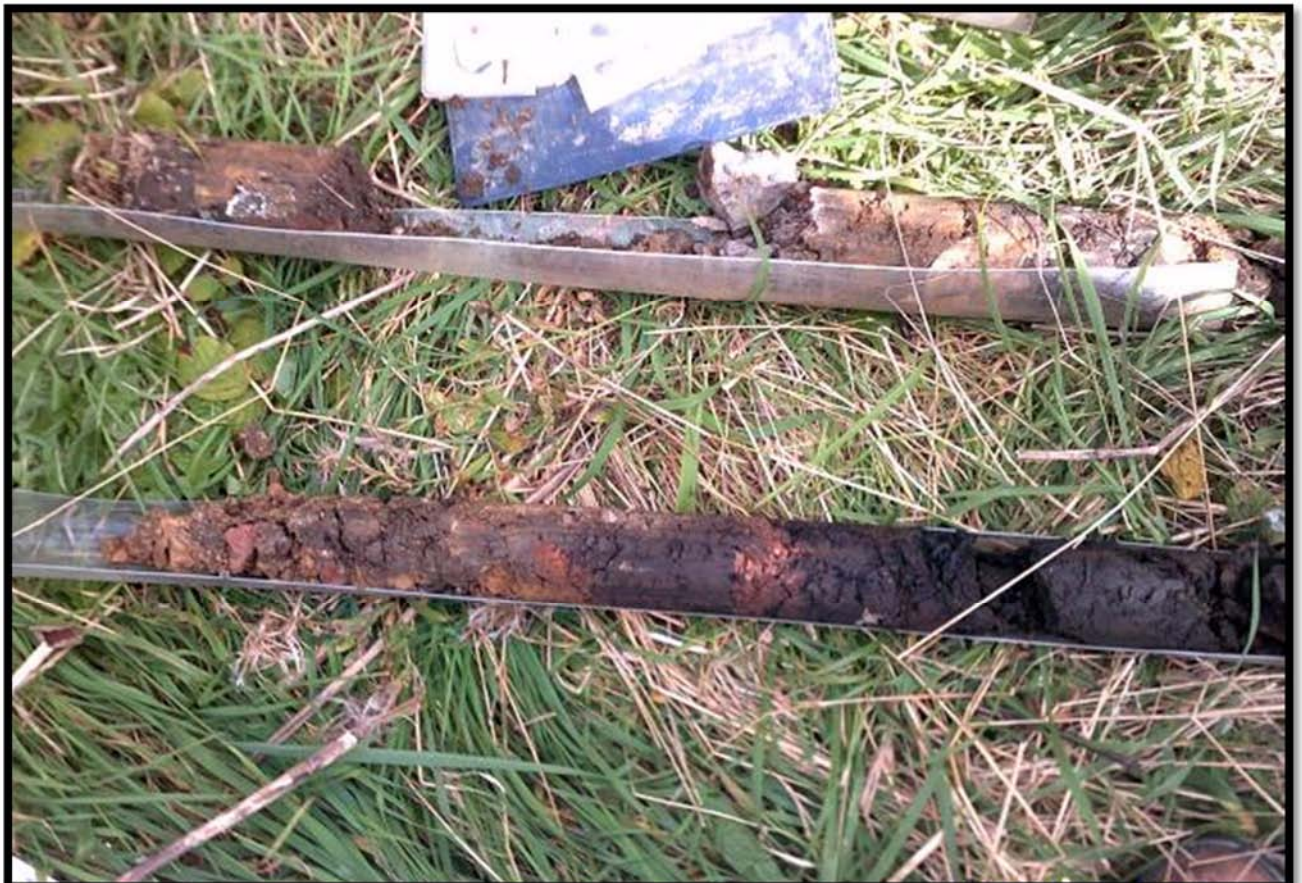
Y: Made ground below WS05
