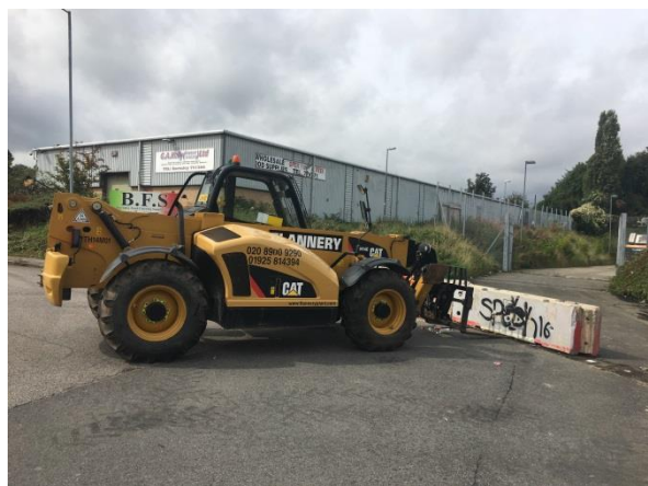
No.6 Telehandler moving the jersey barriers every morning and put them back in place at the end of every shift to keep site secure.
