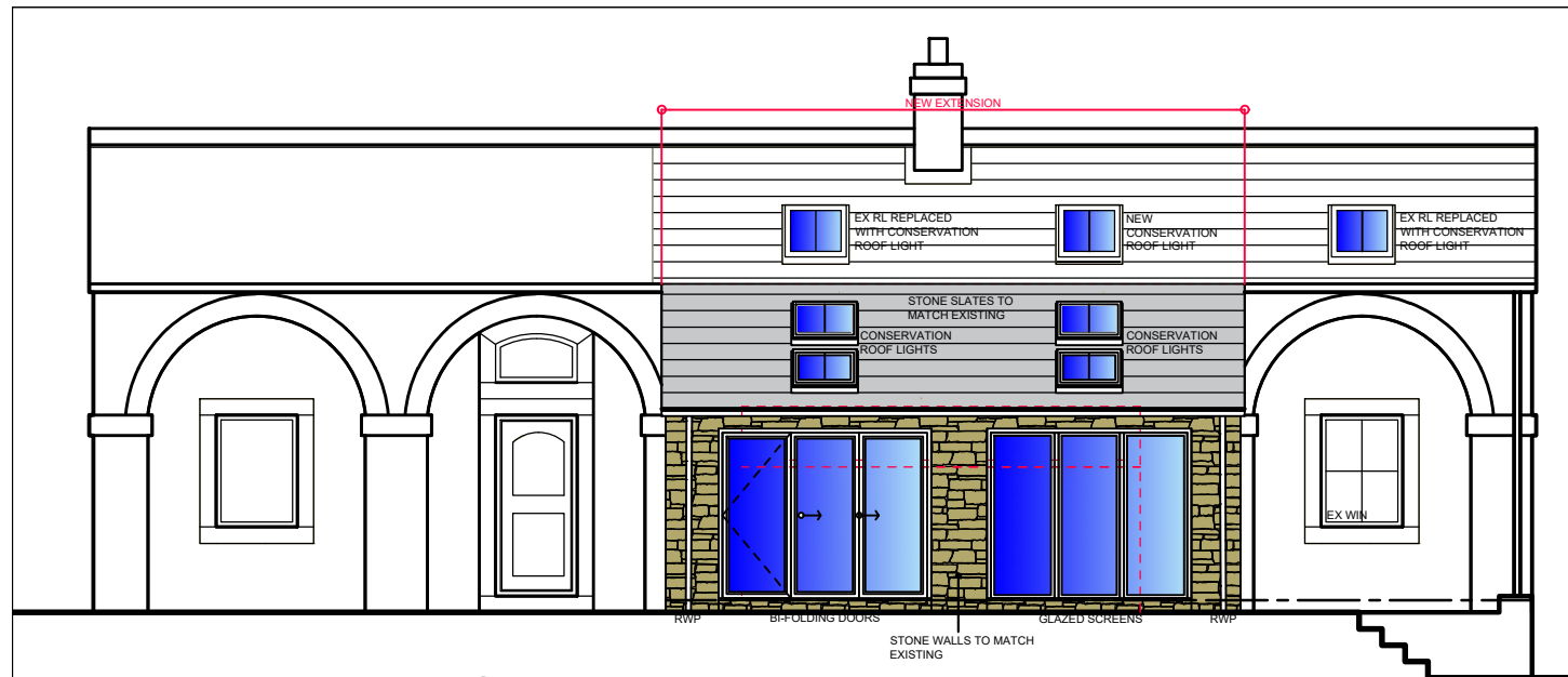
REAR ELEVATION SCALE 1:100
