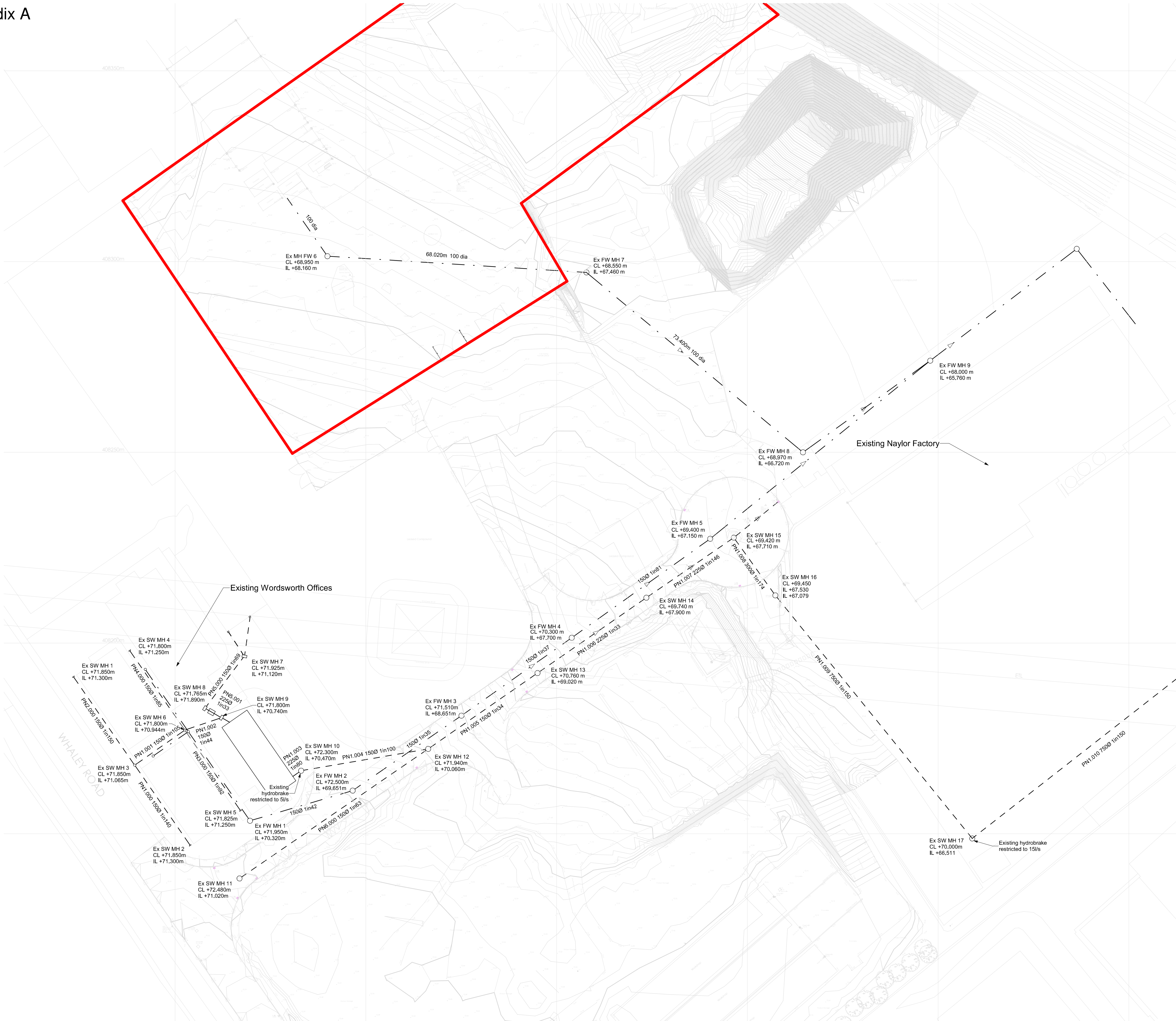
1 Existing Drainage Layout 1 : 500
