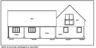
WEST ELEVATION, ENTRANCE & CAR PORT
