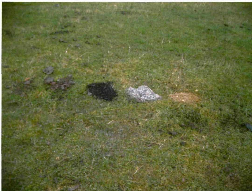
Photograph Number 15 showing the strata drilled through, left side, inert rubble, then coal, light grey fireclay, ganister stone.
