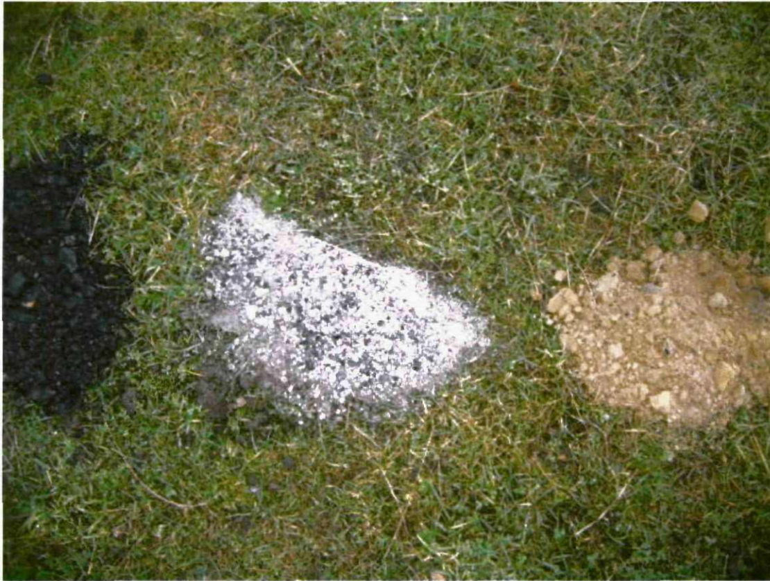
Photograph Number 17 showing the Halifax Hard Bed coal and the fireclay bed above the ganister.
