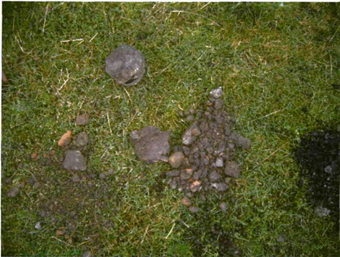
Photograph Number 19 showing the waste drilled through which is stone, brick, earth and concrete.
