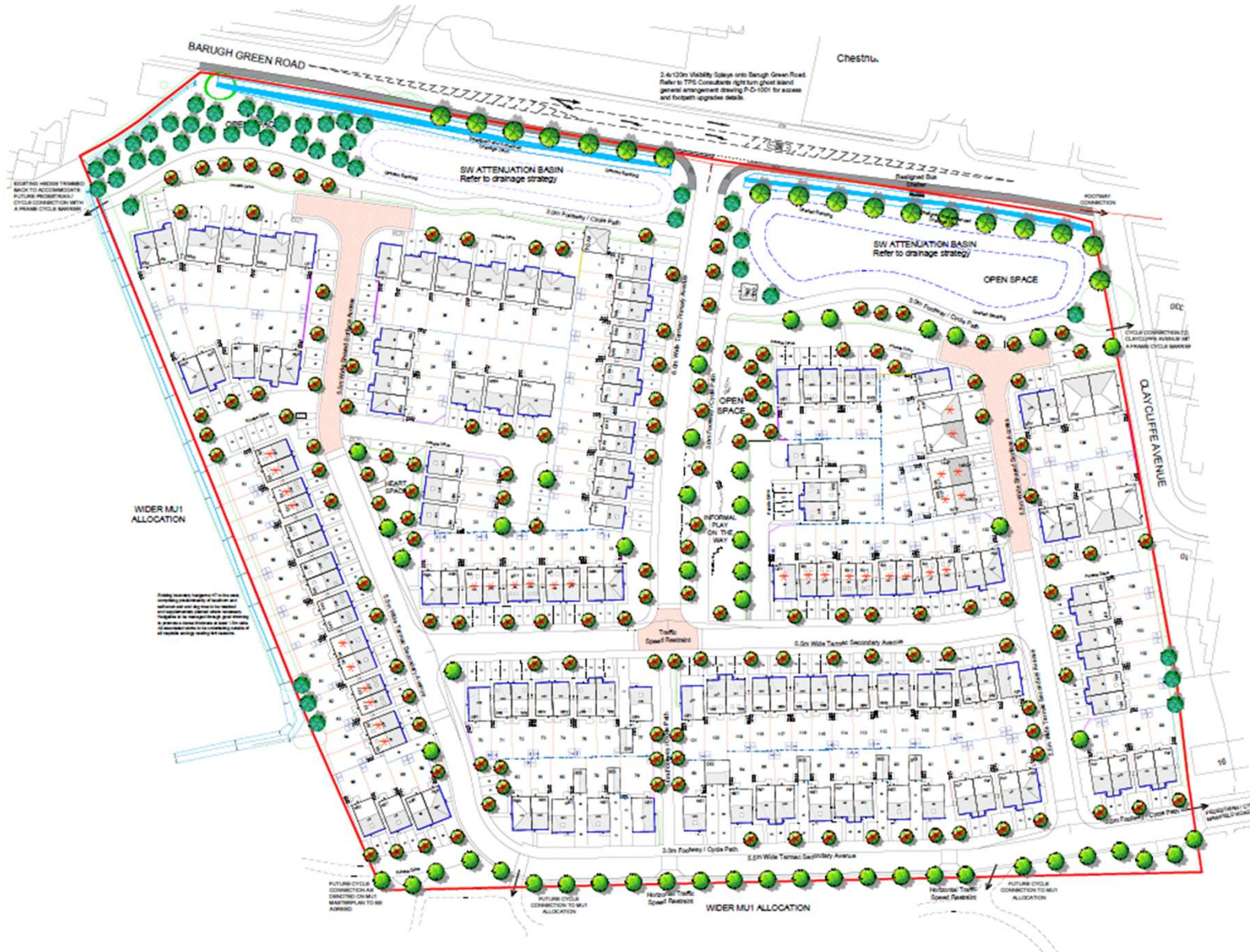
Proposed plan showing the active frontages of the designed scheme to help design out crime.
