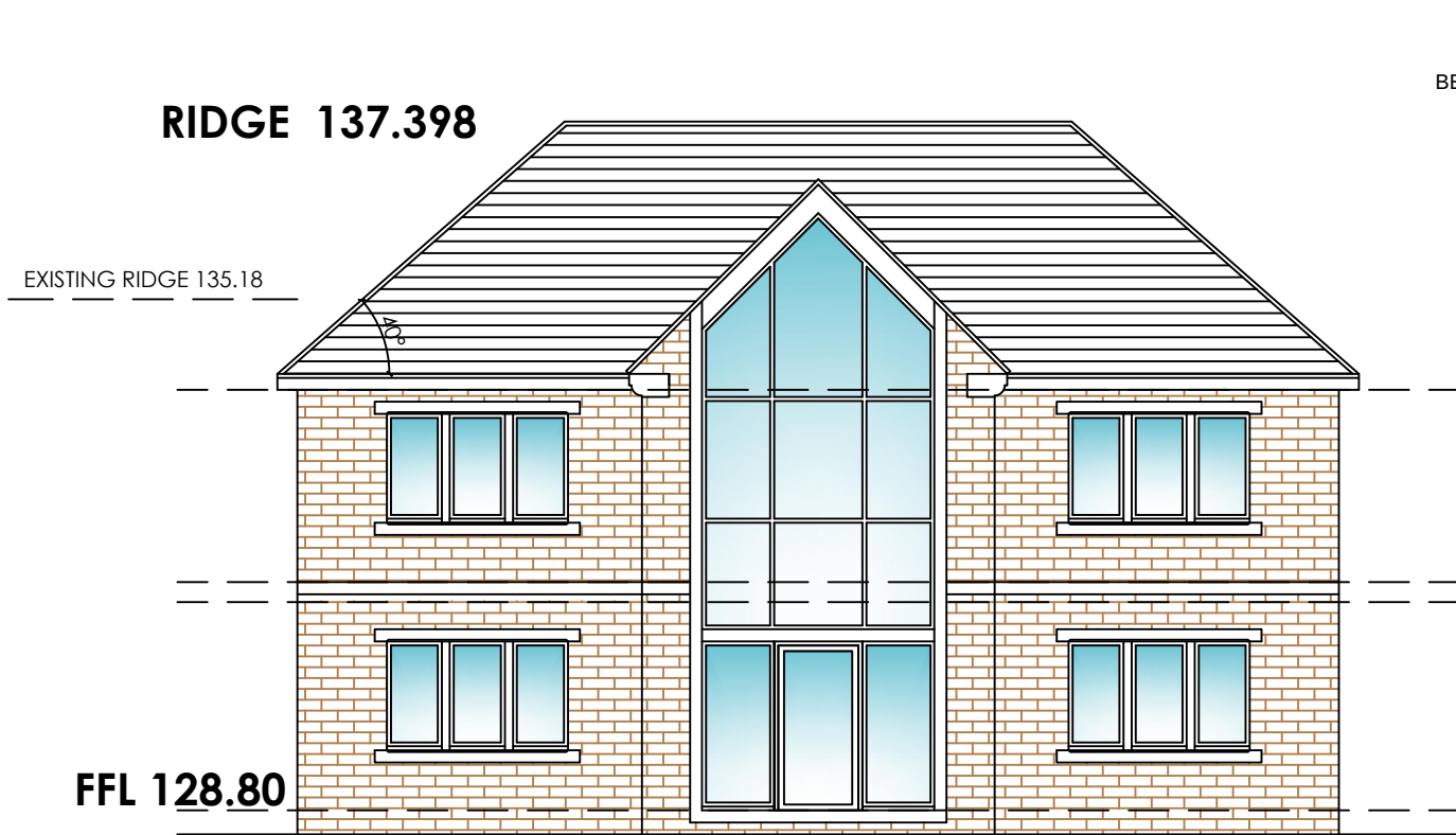
PROPOSED FRONT ELEVATION (SOUTH) SCALE 1:100
