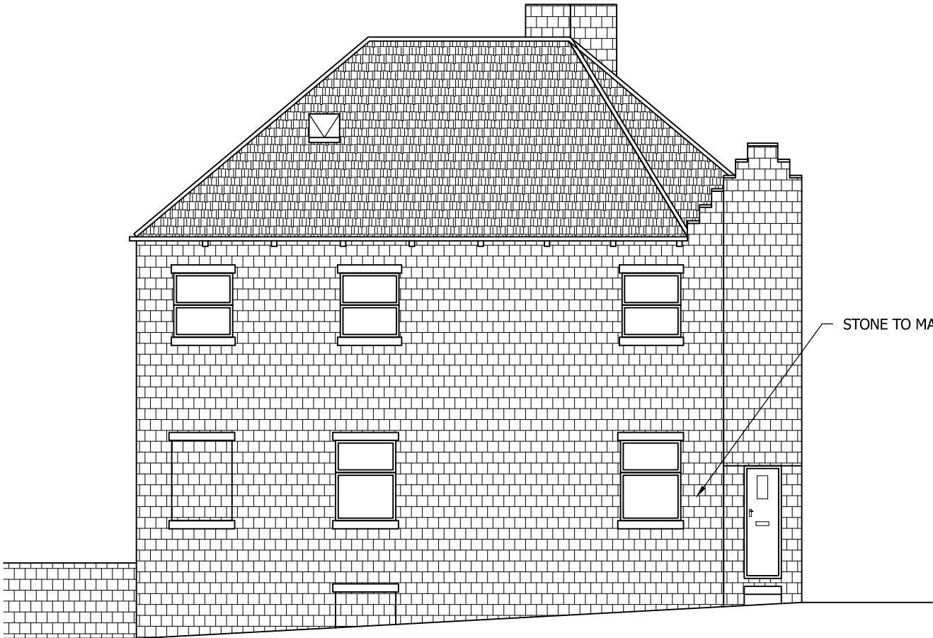
PROPOSED SIDE ELEVATION SCALE 1:100 AT A3
