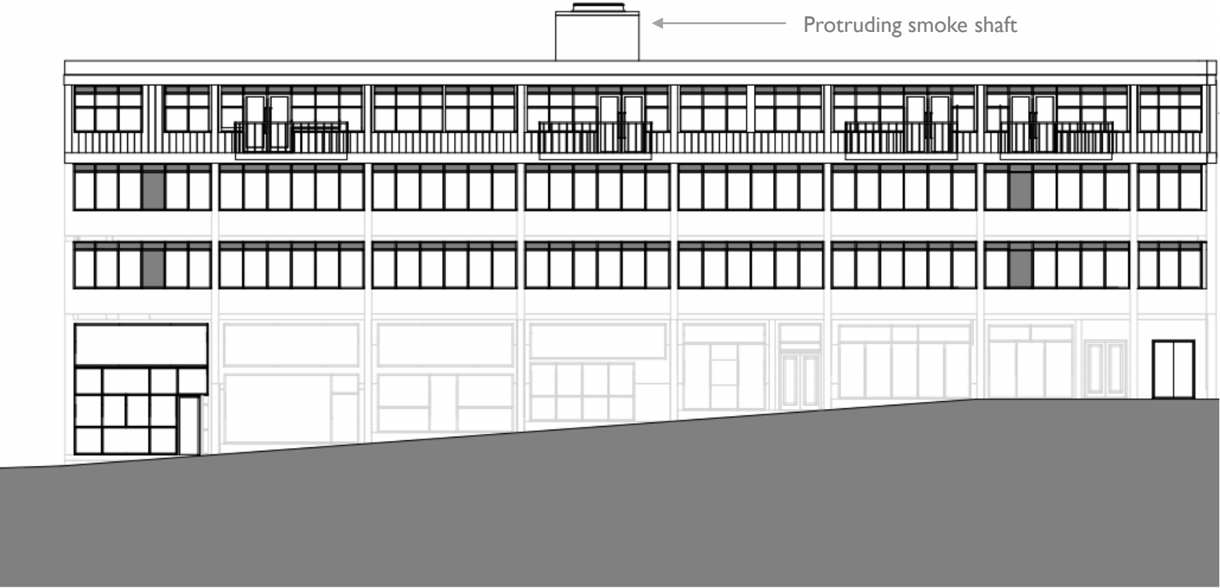
Figure 20 - Front Elevation (Roof Extension) Proposed
