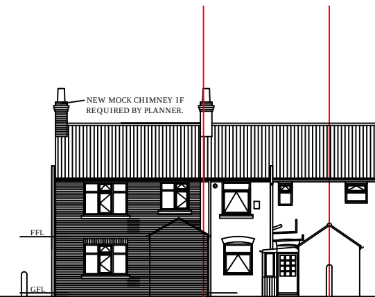
PROPOSED REAR ELEVATION SHOWING NEW HOUSE
